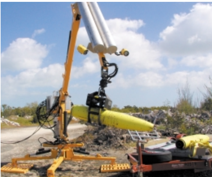
Underwater Ordnance Recovery Inc. non-destructive Bomb Recovery System undergoes a function test prior to being lowered into the water.
